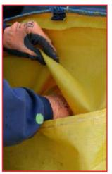
**8.** Should this not be the case, deflate the liner slightly and adjust by pulling the liner through the access overlap flap at the far end of the liner.
