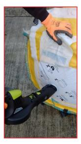
Insert the Inflator through the valve and inflate with the Inflator at maximum.
