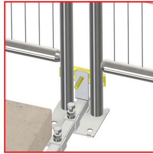
9. Fit back half of gripper coupler into middle Windbreaker base.
