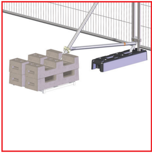
13. Load required number of block on tray.
