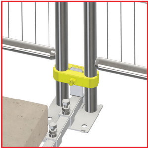
10. Fit front half of gripper coupler and tighten up.
