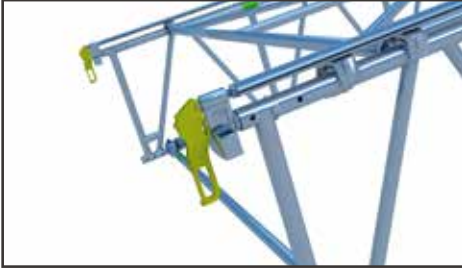
7 Install Track Compressors
