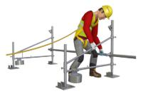
4. Install 48.3mm diameter Glavanised or Alloy scaffold tube to half coupler fittings, to provide 2nd handrails.
