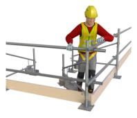
6. Corners can be achieved by connecting lapping tubes 50m offset using regular scaffold double couplers. Set out a further frame 3m from supported corner and continue as step 5.
