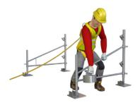
3. Install Safeguard weight on each frame inboard between inside foot and frame bar.
