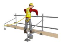
5. Progressively join tube with scaffolding sleeve couplers at the two handrail heights. Safeguard feet have a facility to accept regular scaffold boards to be used as a toeboard as required.
