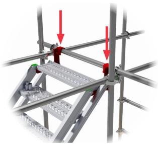
Step #2 – From a safe working level, tighten the integrated anti-uplift bolts on the underside of the tube connector brackets, using a standard scaffold spanner.
