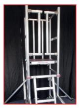
**9.**Using the ladder, climb onto the podium platform
