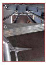
**6**.Fit podium stabilisers at a 45-degree angle (see photo A) Unless against a wall (see photo B) Making sure stabiliser is located on the floor.
