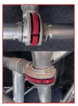
**4.**Position ladder on to lower rung and push down making sure ladder hooks are locked within the guides. Now do the same to the top of the ladder.
