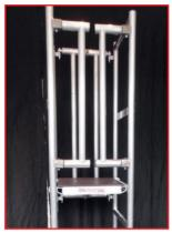
8. Move the gate from the locked position and secure it behind you. Make sure it is locked, never use the podium without locking the gate
