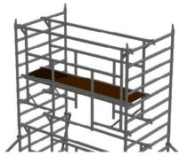
4 Place a trapdoor platform at the appropriate level between the BetaGuard® frames.
