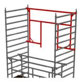
Attach one BetaGuard® frame at outside edge between tower frames at 2nd and 8th rungs.
