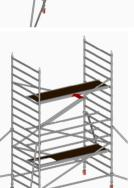
Fit horizontal braces to both sides of platform at 2nd and 4th rungs above platform level to form guardrail protection to single platform only.
