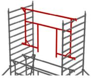
Attach one BetaGuard® frame to centre of tower at 2nd and 8th rungs.
