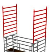
Add two 8 rung frames on top of the existing frames.
