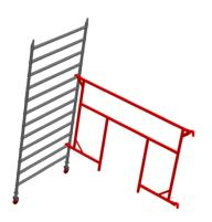
Raise combined frames (ensuring that castors are locked) and attach the BetaGuard® frame at 2nd and 8th rungs of lower tower frame.
