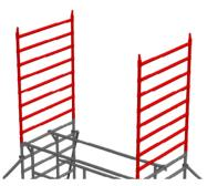
1 Add two 8 rung frames on top of the existing frames.
