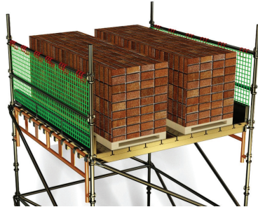
Six No. 8.5kN (0.85 Tonne) 0.8mx0.8m Small pallets (Gates omitted for clarity)
